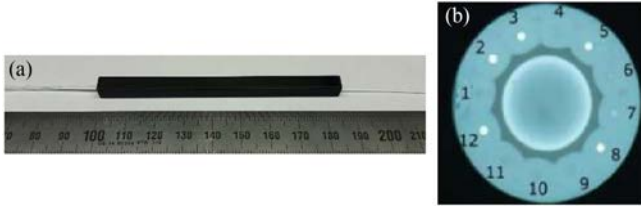
Fig. 2. (a) Packaging of the combiner/fan-in spliced to the 12c-EYDF - (b) Cross view of the bundle.
